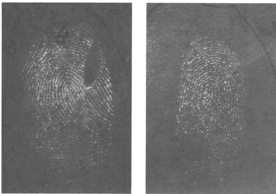
FIG. 1—Fluorescent impressions of latent fingerprints after development with NBD derivatives. Latents were taken from an "average" donor and developed 24 h after stamping. Development from white paper. NBD-chloride (I): (left) solution development and (right) vapor phase development (90 to 95°C, 10 min).
