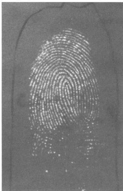
FIG. 4—Same as Fig. 1 except for NBD-OPh (VI): vapor phase development (60 to 65°C; 7½ h).
